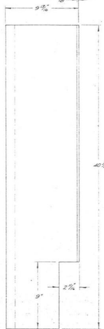
-40R FRONT INNER HORN PANEL, RIGHT - 1 REQD (SHOWN) -40L FRONT INNER HORN PANEL, LEFT - 1 REQD (OPPOSITE)
